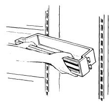
To **remove bins:** Lift bin straight up until mounting hooks disengage.
